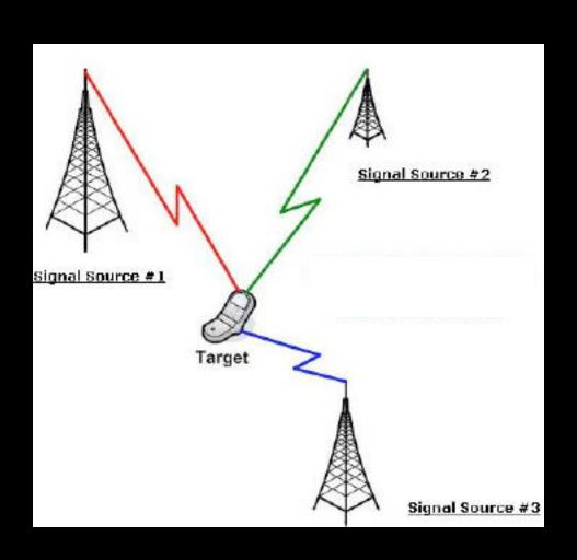
triangulation of radio signals (GPS, WiFi, RFID, TV/radio)
