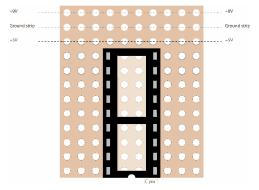
Place the IC socket on the board so that the pins fall exactly over the part where is no copper on the other side.
