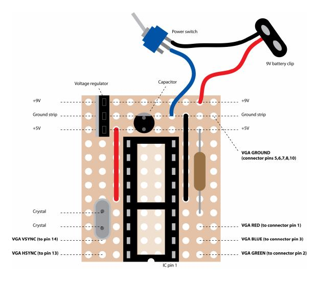
Now it is time to program the microchip and put it into place. Make sure you put it the right way: it has a slight dent on one short side that should align with the dent in the IC socket (see picture).
