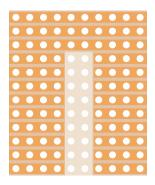
The board has on the copper side a strip in which the copper has been taken out.
