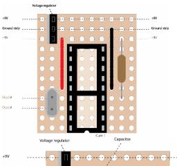
Place the crystal and solder it to the board. The direction does not matter.
