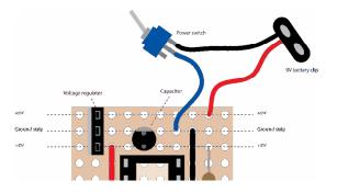
Strip a blue wire and solder it to the ground strip as well. For steadiness, the wire can go through the hole of the 7805 regulator.
