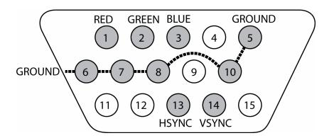
First, put solder in all pins that are grey. Heat the pin a little and let a little solder flow into the pin. This will help you connecting the wires later more easily.
